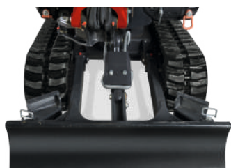
Retracted undercarriage : 980 mm
