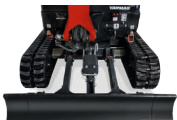
Extended undercarriage: 1320 mm
