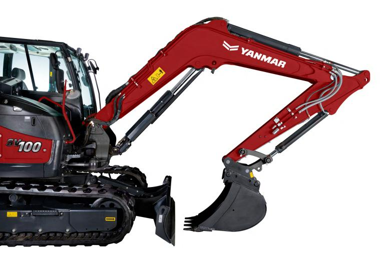
Designed with reliability in mind, the SV100-2 is robust, durable and capable of delivering demanding work – even in the toughest conditions and most challenging terrains. The structure of the undercarriage, alongside heavy-duty steel covers, effectively protects the chassis against daily damage and minimises unnecessary downtime. Hoses come as standard with abrasion-resistant sleeves, while their position on the top of the boom further reduces the risk of torsion.
